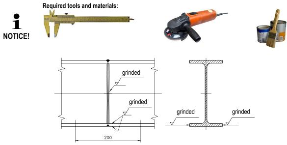
Fig. 1: Smoothing of welded track beams
