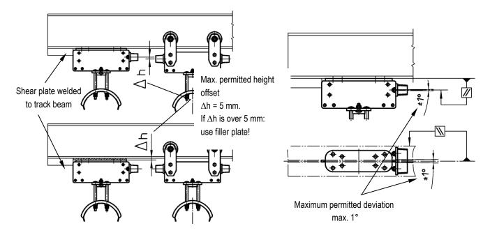
Fig. 24: Mounting the end clamp
