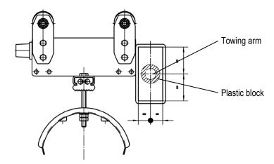
Fig. 23: Orientation of the towing arm
