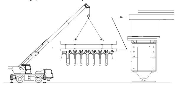
Fig. 21: Mounting a pre-assembled festoon system
