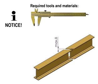
Fig. 3: Girder joint for non-welded track beams
