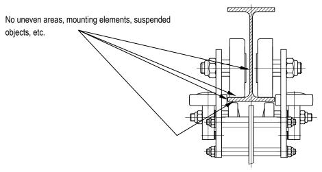
Fig. 2: Use of even welded track beams
