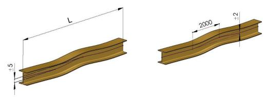
Fig. 6: Vertical deviation of track beams
