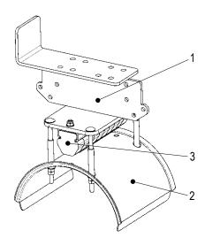
Fig. 13: Towing clamp
