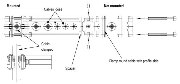
Fig. 29: Mounting round cable clamps
