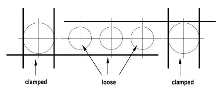
Fig. 30: Schematic diagram of preparation for installation of round cable clamps
