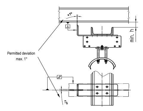
Fig. 22: Mounting a towing clamp
