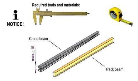
Fig. 8: Poor vertical alignment between the crane beam and track beam
