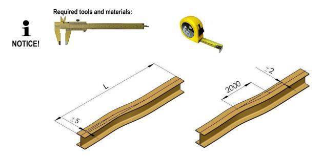
Fig. 5: Horizontal deviation of track beams, L = total length
