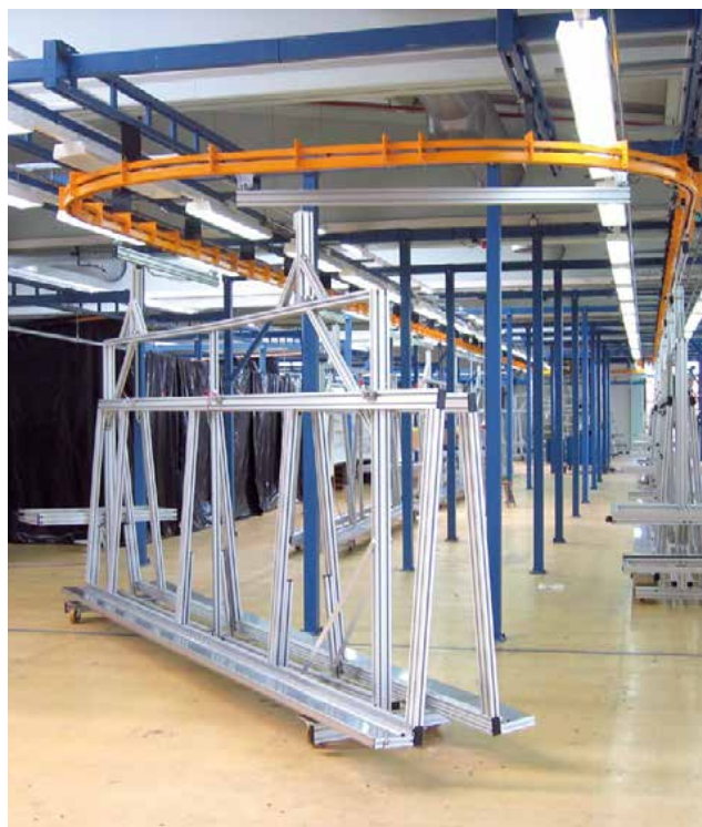
Power & Free system for the assembly of customer-specific wiring harnesses
