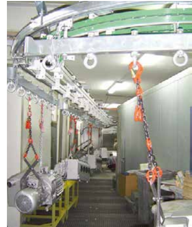
Overhead monorail system combined with a loop-conveyor for the transport of vacuum pumps through a drying furnace
