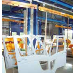
Overhead monorail system for the manual transport of vehicle components
