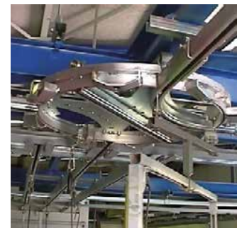
Turning switch For the regulation of material flow at intersection points; manual or pneumatic
