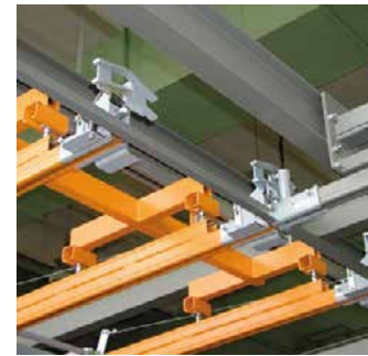
Sliding bridges For cross-line transport when supplying individual tracks in a painting and drying area
