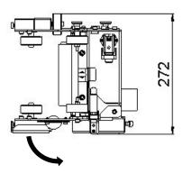
Lower part of the running gear can be folded down
