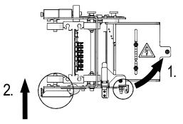
c) Open the lower flap of the trolley using the two fasteners (right and left on the trolley).
