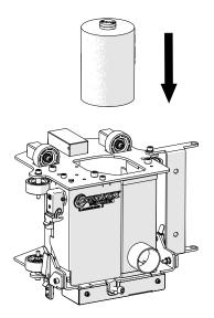
Circular brush must be guided easily onto the pin and then turned into the correct position.
