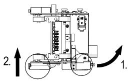
b) Open the lower flap of the cleaning head using the two clamping locks (on the right and left of the trolley).
