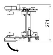
Lower part of the running gear can be folded down
