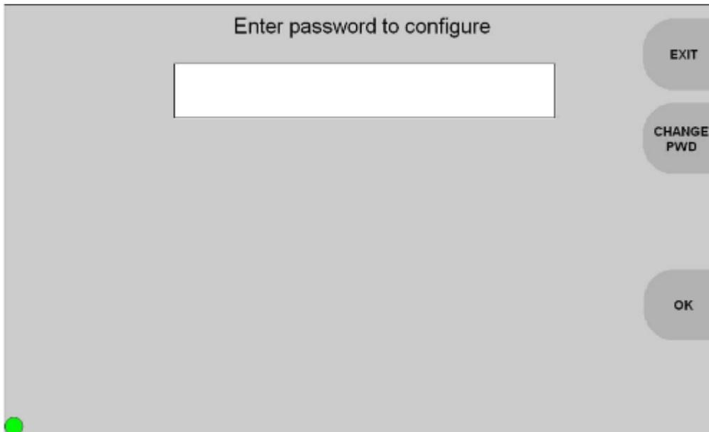
To enter a password, select the password to be enter with key UP or DOWN use keys PUSH to edit and validate the password, UP and DOWN to choose the character and LEFT and RIGHT to select the cursor position (for further information see chapter 6.3.1).
